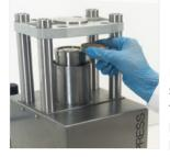
Position the sample and the roughened plate in the press.
